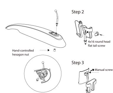
1, Use the M5 Allen key to lock the Hand-controlled hexagon nut to the remote control bracket.
